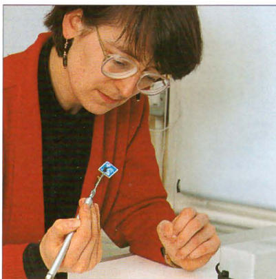
Using the vacuum tweezer
